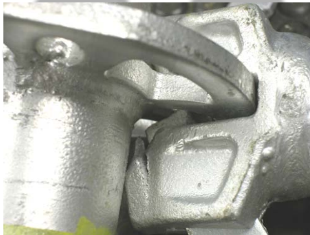
Failure of wedge at 14,173 lbs.
