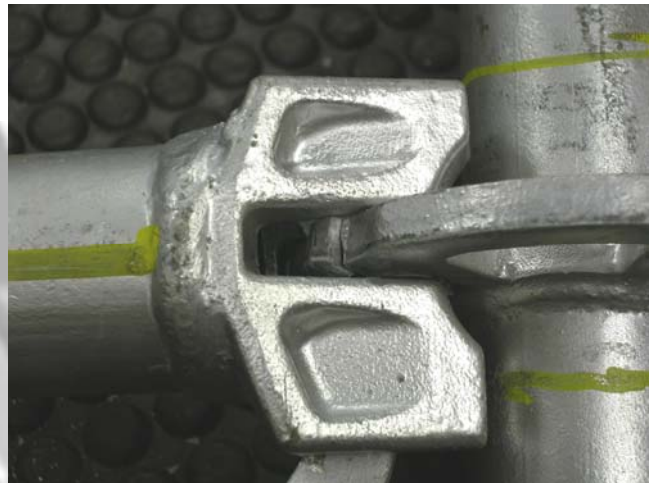
Failure of rosette at 111,811 lbs.
