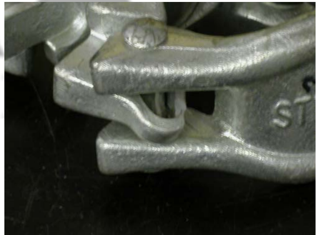
Swivel #2, failure of forging around pivot pin
