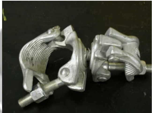
Swivel #1. Ultimate failure at 16,000 lbs.
