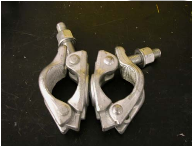
Swivel #2. Ultimate failure at 9,779 lbs.
