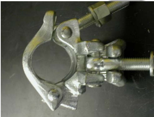
Right angle #2. Ultimate load of 15,150 lbs.
