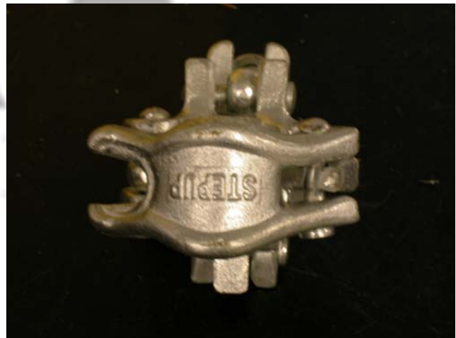
Right angle #2. Deformation of pivot pin, and forging around pivot pin
