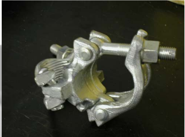
Right angle #1. Ultimate load of 14,580 lbs
